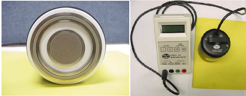
Figure 3.6 Concentric ring electrode and electrode setup
