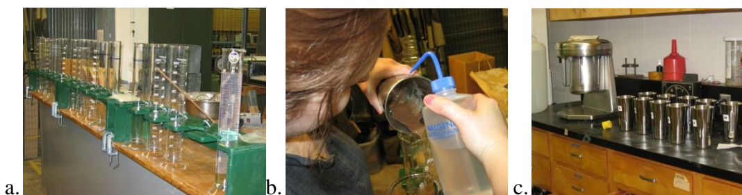
Figure K.3. (a) graduated cylinders used in analysis (b) transferring agitated samples to graduated cylinders and (c) mixing apparatus used to agitate samples before transferring to graduated cylinders.
