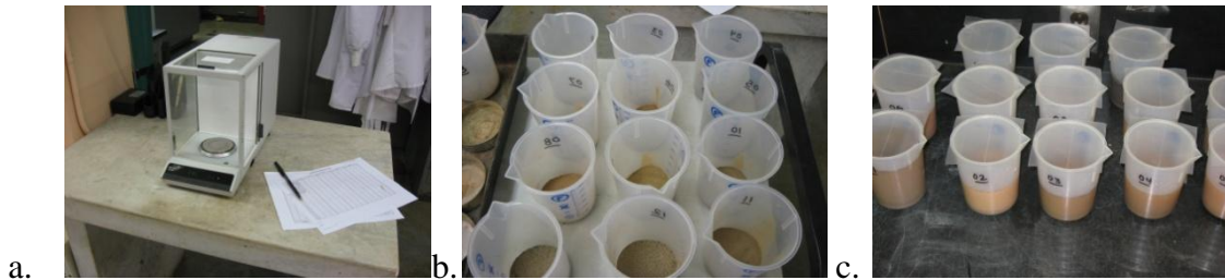
Figure K.2. (a) scale used to weigh samples (b) plastic beakers used for holding samples, and (c) samples covered in parafilm prior to being placed in graduated cylinders for analysis.
