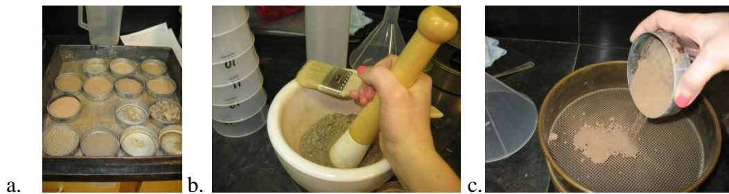
Figure K.1. (a) samples after oven drying, (b) grinding of samples using mortar and pestle, and (c) sieving of samples to remove gravel portion.
