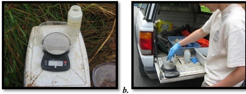
Figure G.3. (a) Photo displaying field scale zeroed between samples (b) photo of sediments being weighed
