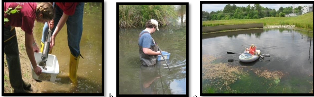
a. Figure 4.2. Photos of sediment collection procedure (a) steel auger used in sediment sampling (b) floatable bins used in collection (c) inflatable raft used for sampling when forebay was not wadeable.
