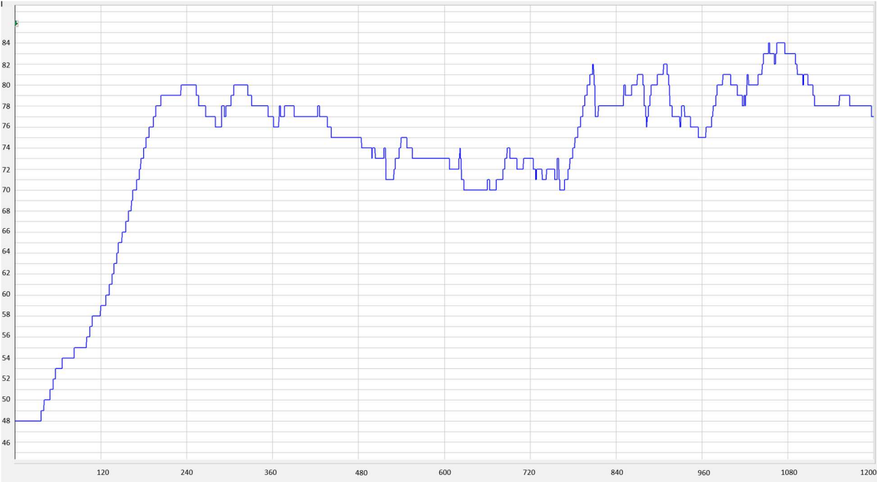
Figure 22. Engine coolant temperature (°C) vs. time (s) in Trial 5.
