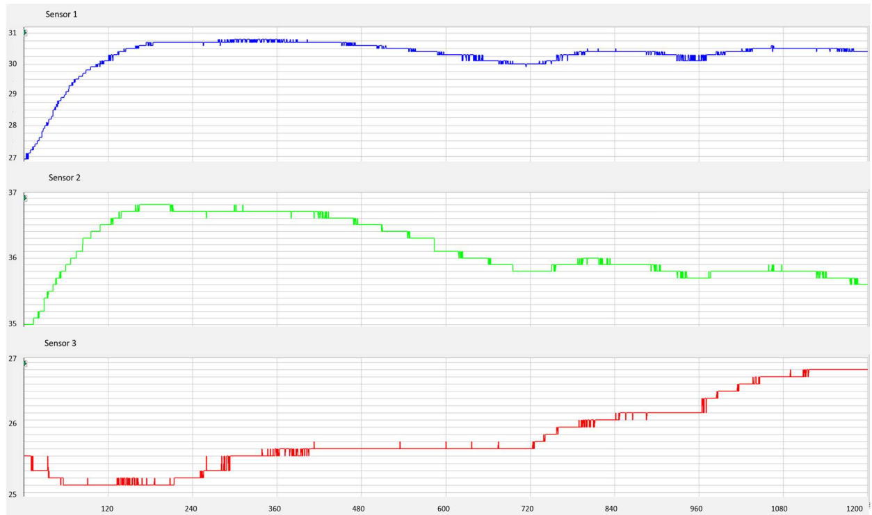
Figure 17. Battery temperatures ( ^{\circ}\text{C} ) over time (s) for second run with diversion (T5).
