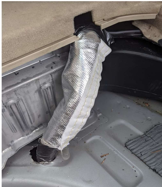
Figure 12. Exhaust transport hose feeding into battery compartment.
