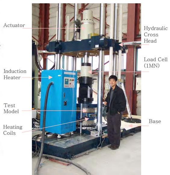
Fig.2 Creep-fatigue Test Facility
