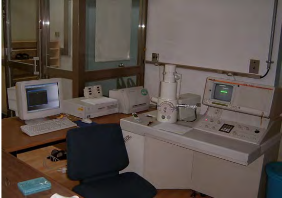
Fig.6 Scanning Electron Microscope (JEOL)
