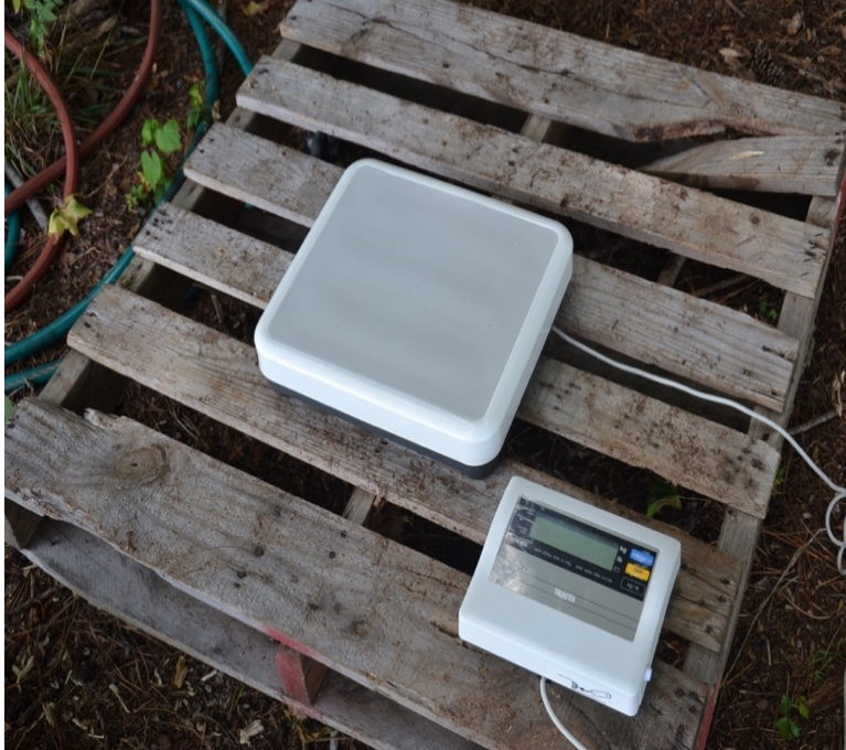
Figure 7 Scale used to weigh mushrooms in the field. The scale was set on a flat surface to ensure that it remained in balance.
