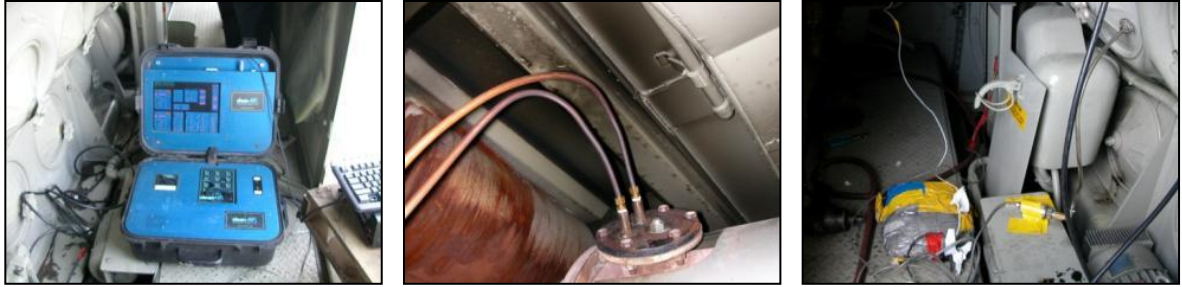
Figure 2-5: Installation of PEMS on an F59PHI Locomotive Prime Mover Engine (a) PEMS main unit (front-view); (b) exhaust sampling port and metal tubes; (c) sensor array box
