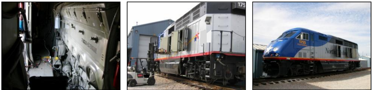
Figure 2-7: Installation of PEMS Exhaust Sample Lines in an F59PHI Locomotive (a) routing sampling hoses and cables; (b) routing sampling hoses through a side door, secured with ties (rear-view); (c) side-view of F59PHI locomotive
