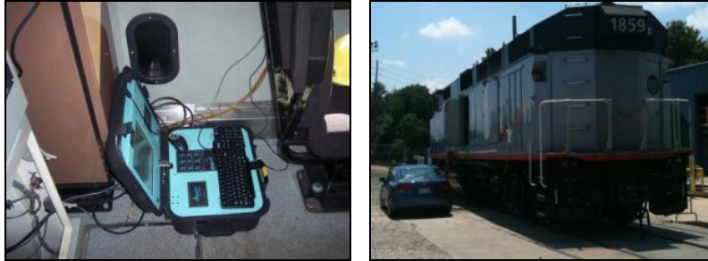
Figure 2-2: PEMS Placement for F59PH Locomotive Prime Mover Engine Measurement (a) inside of the locomotive cab; (b) inside an air conditioned vehicle during extreme heat
