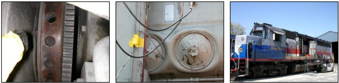
Figure 2-9: Installation of Sensors on a GP40 Locomotive Prime Mover Engine (a) RPM sensor; (b) manifold absolute pressure (MAP) sensor; (c) side-view of locomotive
