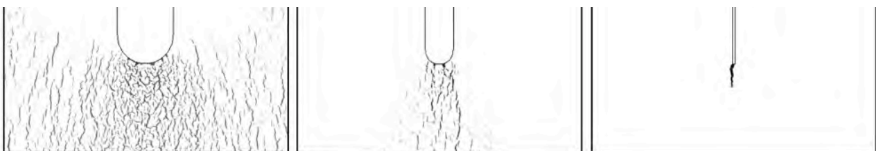
Figure 3. Theoretical predictions of hydride precipitation at notch and crack tips: notch geometry changes from blunt at the left, to sharp at the right. Average hydrogen concentrations and peak stresses at notches are kept the same for three cases. External tensile stresses are applied in the horizontal direction.
