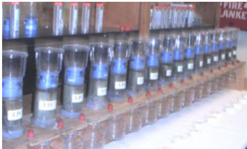
Figure 2. Soil columns instrumented with the Nalgene funnel on the top of column and leachate bottles at the bottom of column.
