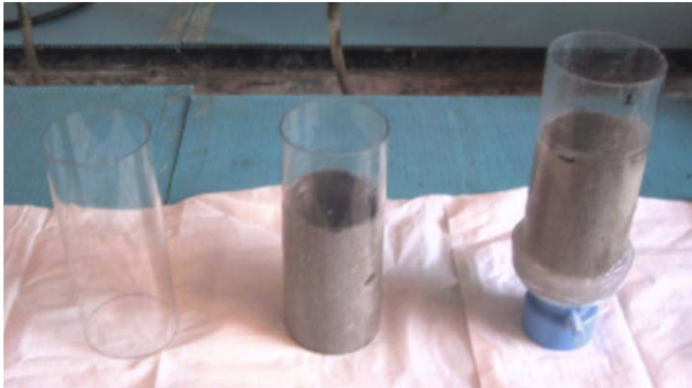
Figure 1. Sand coated PVC liner and sealing to the Nalgene filter unit. From left, a clean PVC liner was coated with the study soil (coated at < 1-mm thickness) and then sealed with Nalgene filter unit for column leachate collection.
