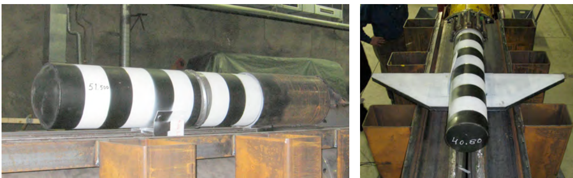
Figure 5. An aluminium pipe missile (left) and a non-axisymmetric missile with wings (right).
