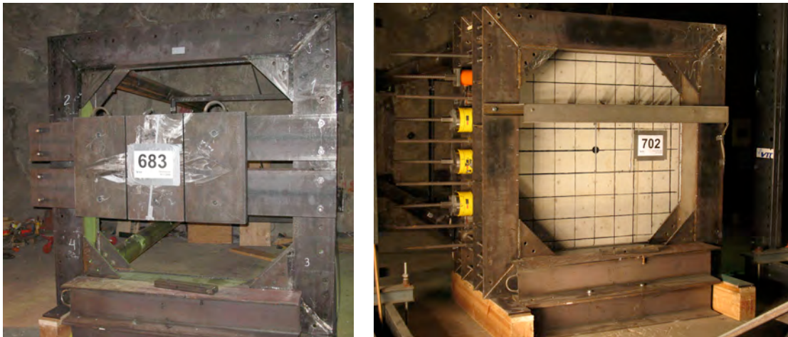
Figure 4. Rigid-like steel plate for measuring impact forces (left) and deformable concrete wall (right).
