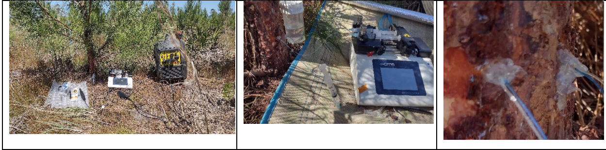
Figure 2.4: Gas-powered generator and microdialysis pump was set up next to each tree after removing the flammable substrate from around the generator. (Middle) The microdialysis system consisted of four syringes and four microdialysis probes drilled into the tree after carefully removing the outer layer of bark. (Right) Each hole was flushed with DI water and sealed using silicone paste to prevent leaking.
