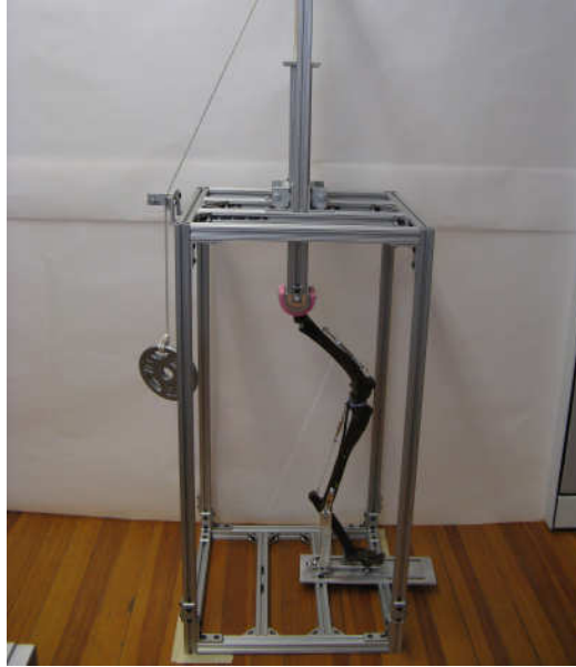
Figure 1.5.38: Testing fixture with assembled leg fixed for testing.
