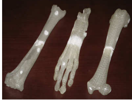
Figure 1.5.22: Quickcast models made from SLA® used for fixture design and visualization.
