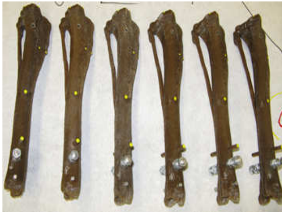
Figure 1.5.31: Tibiae with identically drilled holes at distal end for tarsal joint attachment.
