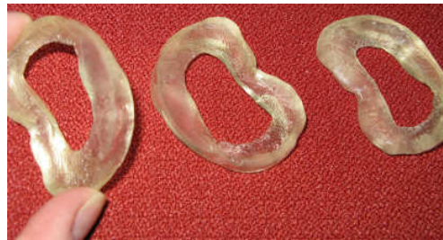
Figure 1.5.27: Three copies of RP menisci built on the SLA® 190 [3D Systems Corp.].
