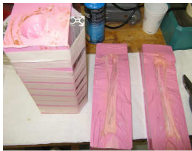
Figure 1.5.25: Tibial mold with glass fibers randomly oriented along shaft.
