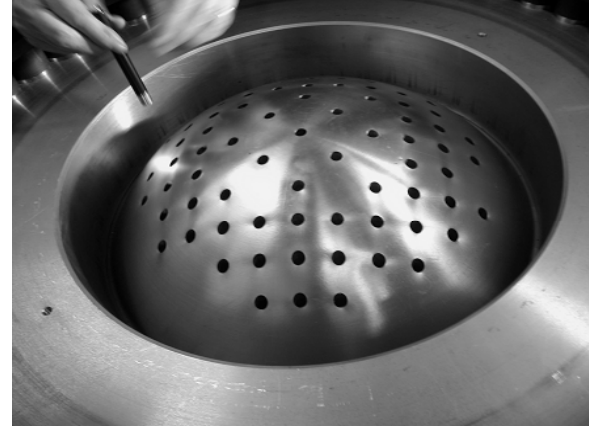
Fig. 7. Specimen EZ1 (small size) after testing, shown with the liner (left). Right: Specimen FB after testing. The test ended due to the failure of the liner.
