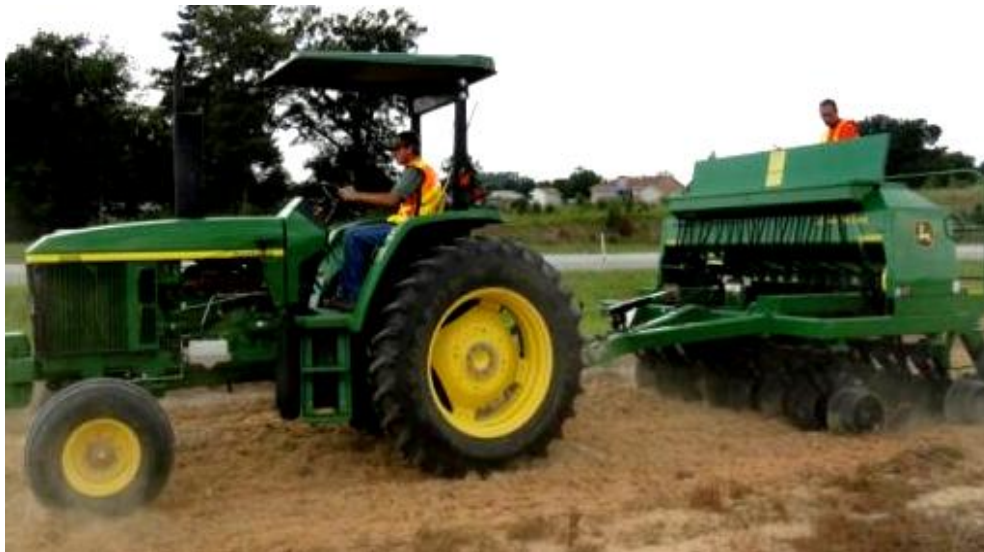
Figure A2.1.2 Planting with John Deere 1590 no-till drill following maximum tillage treatment at Knightdale research site (photo courtesy of NCDOT).
