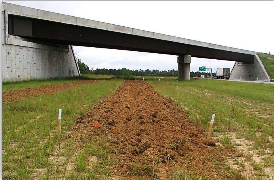
Figure A2.1.3 Seedbed preparation by maximum tillage treatment at Knightdale research site (photo courtesy of NCDOT).
