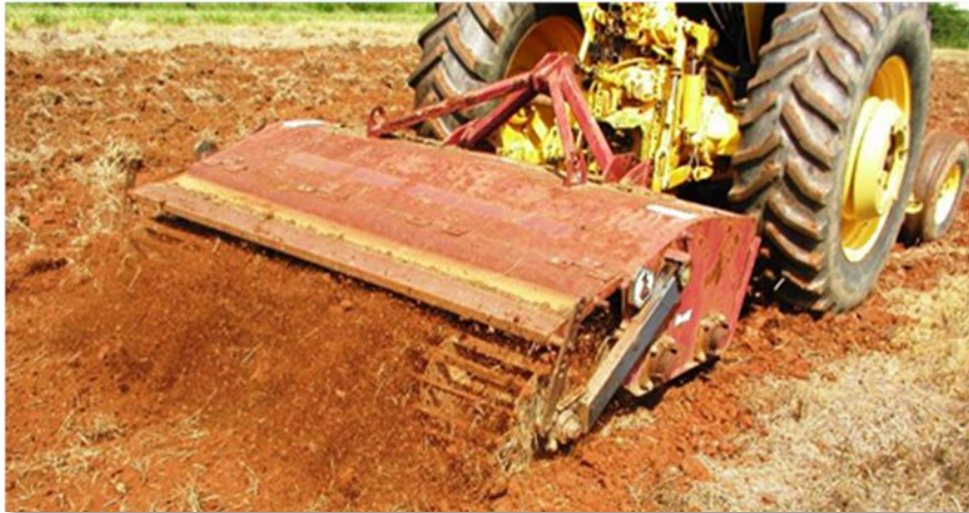
Figure A2.1.1 Rotary tillage with New Holland 6640 tractor coupled with M&W Dyna-Drive surface cultivator (1 pass, followed by planting with no-till drill for minimum tillage treatment; 3 passes, followed by planting with no-till drill for maximum tillage treatment) (photo courtesy of NCDOT).
