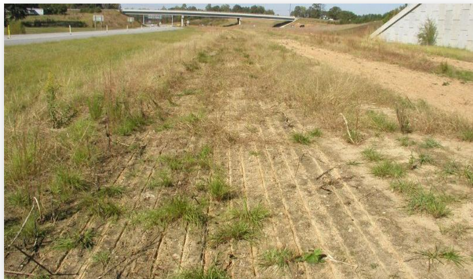
Figure A2.1.6 Depiction of minimal soil disturbance associated with no-till treatment with John Deere 1590 at Knightdale research site (photo courtesy of NCDOT).
