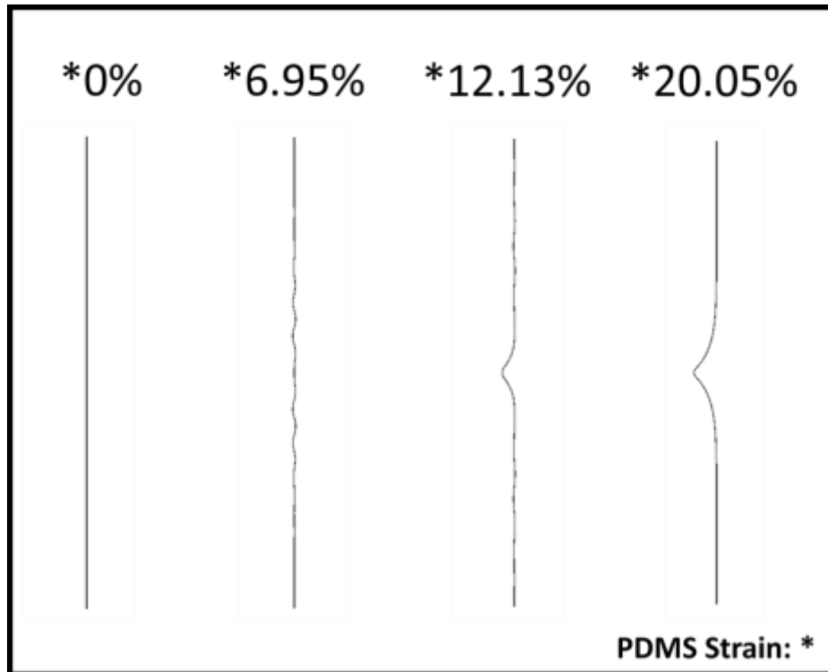
Figure 3.5 Buckling evolution of NW #3 obtained by FEA simulation at specific strain values applied to the PDMS COMPOSITE substrate.
