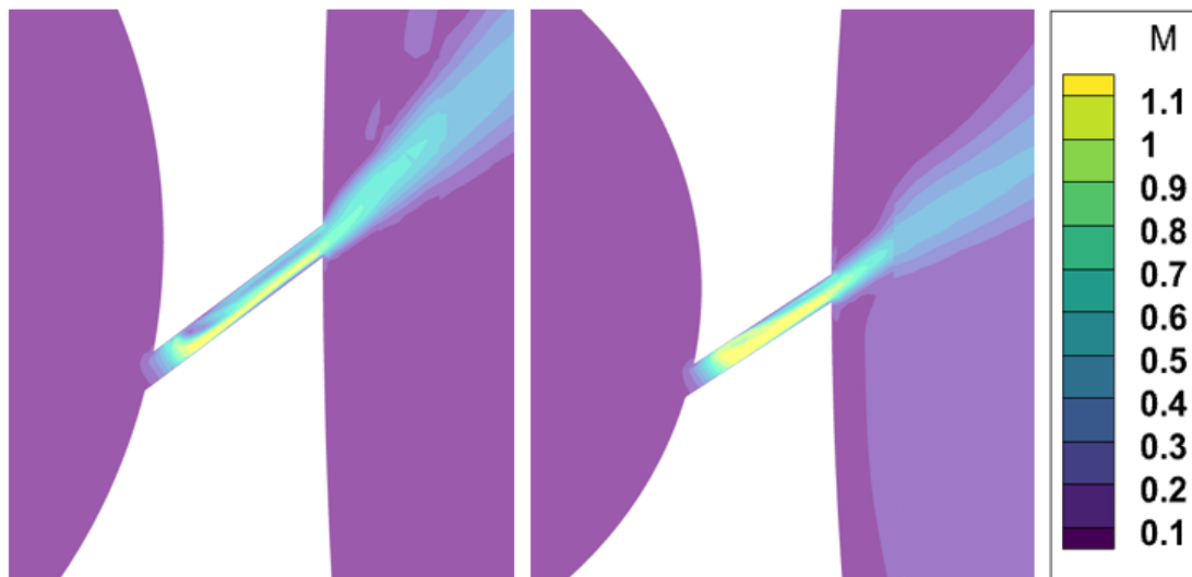
Figure 3.10 Mach contour of the fluid for the 35-degree inclination at 0 RPM (left) and 5000 RPM (right)
