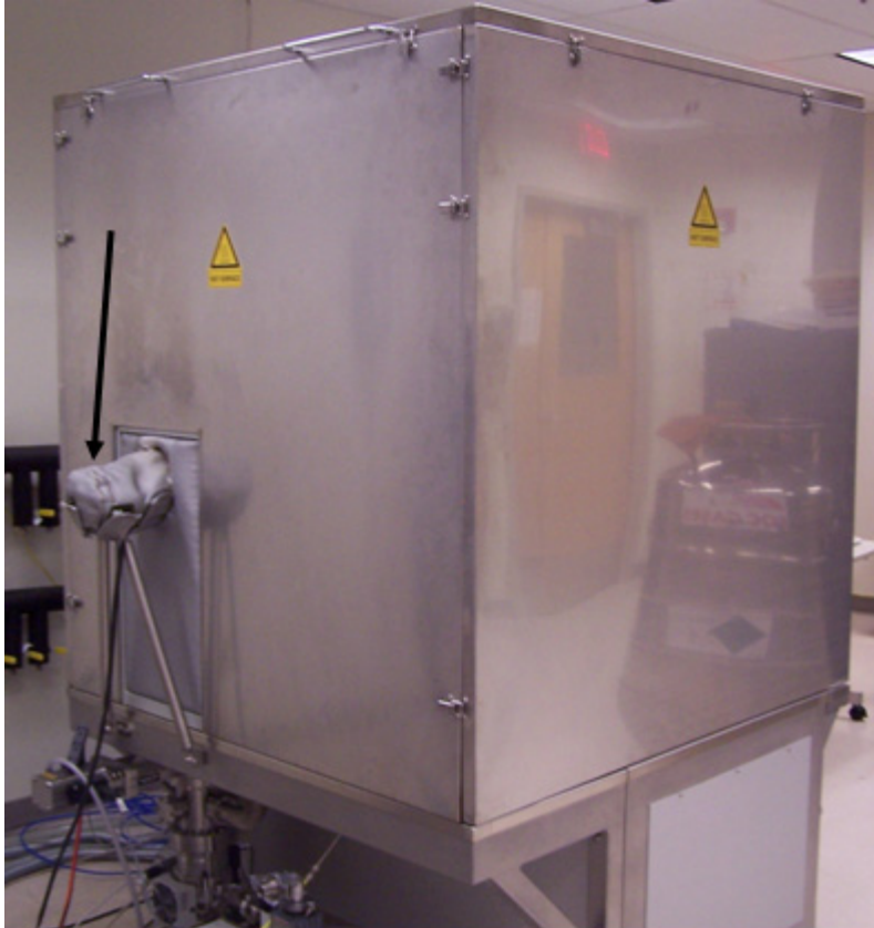
Figure 3.3: Multiprobe P bakeout cover in place. Note that the transfer arm is covered with its own custom insulated cover, indicated by an arrow, because it extends outside of the confines of the bakeout cover. A similar insulated cover is placed on the other transfer arm (with the magnetic probes removed), allowing the transfer arms to be baked with the rest of the chamber.
