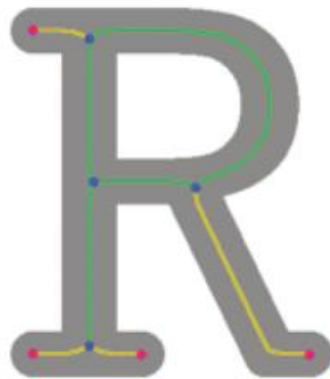
Figure.2.20. Diagram of the skeleton of a feature with five endpoints (red), four nodes (blue), four terminal segments (yellow), four internal segments (green) [47].
