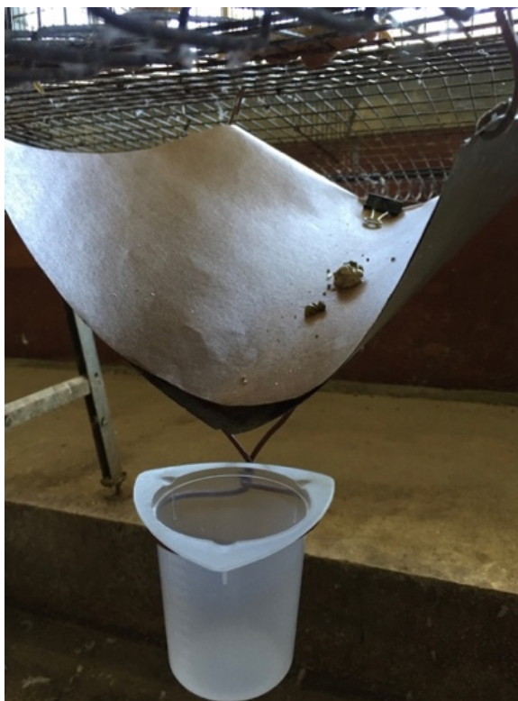
Figure 1. Fecal matter and liquid portion collection pan set up.
