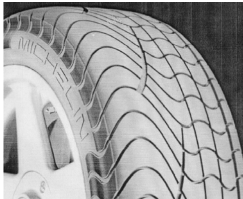
Figure 1.1: A manually carved tire tread pattern [Michelin Americas R & D].
