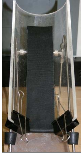
Figure 3.3 Attachment of Material to Gutter with Clips
