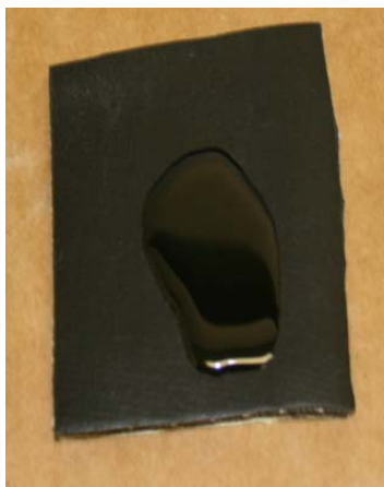
Figure 4.3 m -Cresol on Rubber Sample
