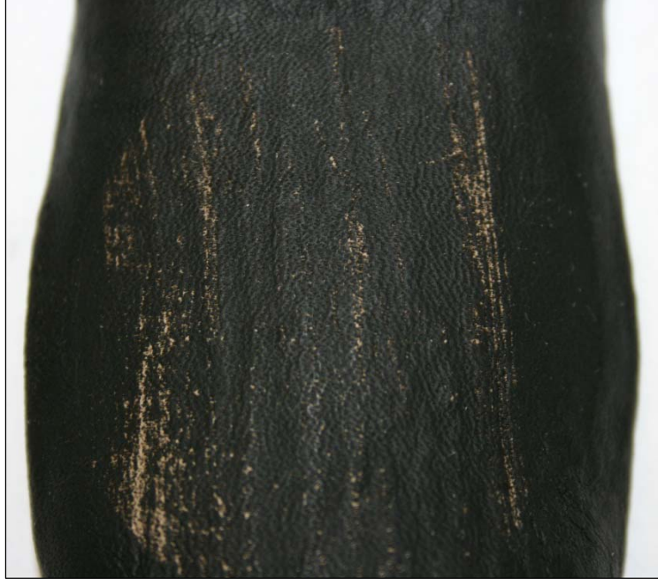
Figure A.2 Leather Sample After Two Minutes with a Rough Brush
