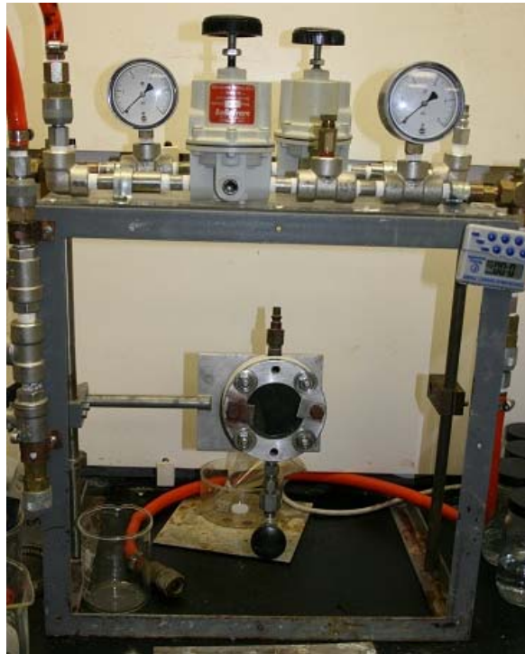
Figure 3.11 Penetration Test Apparatus
