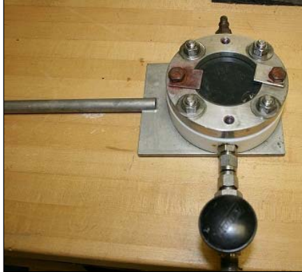
Figure 3.10 Assembled Penetration Cell
