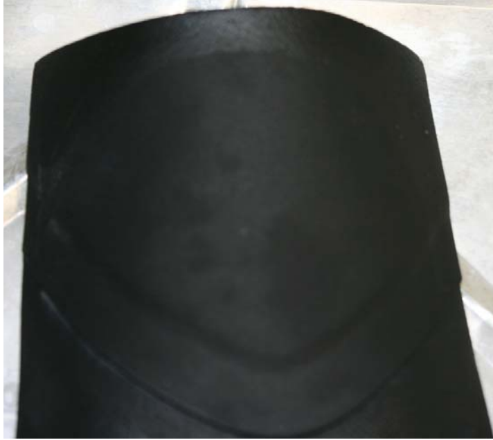
Figure A.3 Rubber Sample After Ten Minutes of Scrubbing with a Sponge
