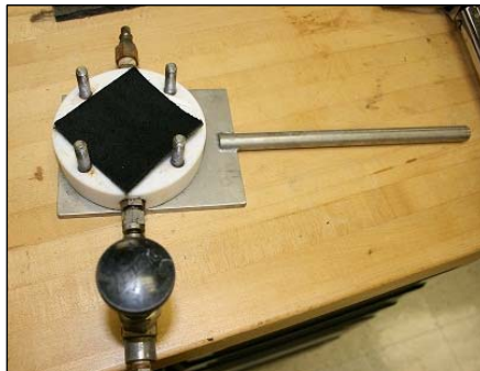
Figure 3.9 Material Sample Loaded into Penetration Cell
