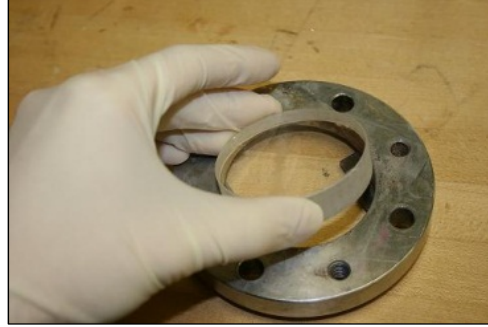
Figure 3.8 Disc Placement in the Restraining Ring of Penetration Cell
