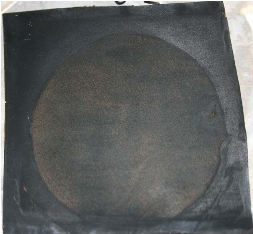
Figure A.4 Leather Sample after Ten Minutes of Scrubbing with a Sponge
