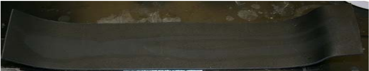
Figure 4.2 Leather Exposed to Modified ISO 6530 Acrolein Splash Test
