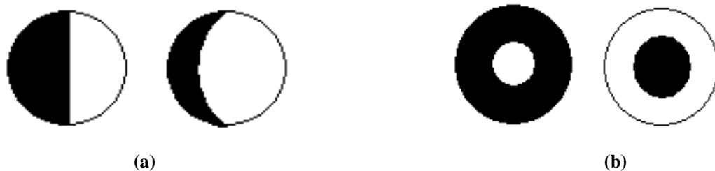
Figure 2.11 Displacement of interface due to viscosity difference a) for Side-by-Side cross section; b) Sheath-Core cross-section [15].
