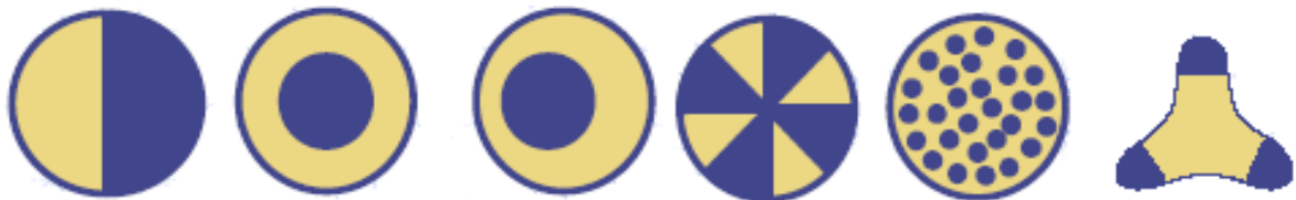
Figure 2.10 (a) Side by Side (b) Sheath/Core (c) Sheath/Core Eccentric (d) Segmented Pie (e) Island in the Sea (f) Tipped Trilobal [14].
