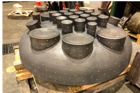
Figure 2. Upper head of the NuScale Power reactor produced at a 44% scale.
