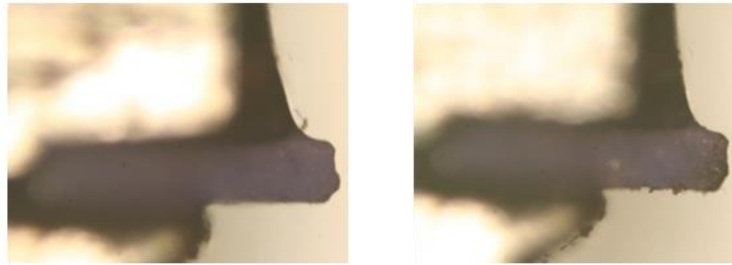
Figure 5-25. Grit Wear Shaping Method: Original (left), after seven passes (right)
