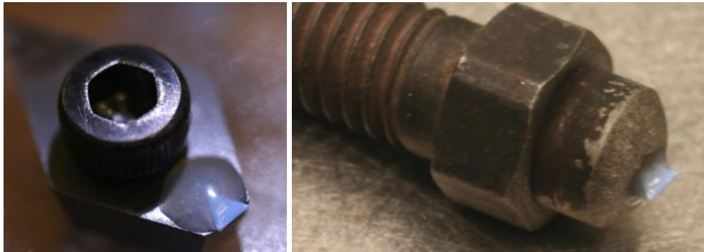
Figure 3-2. Epoxy Mounting on a Flat Surface (left) and in a Notched Hole (right)
