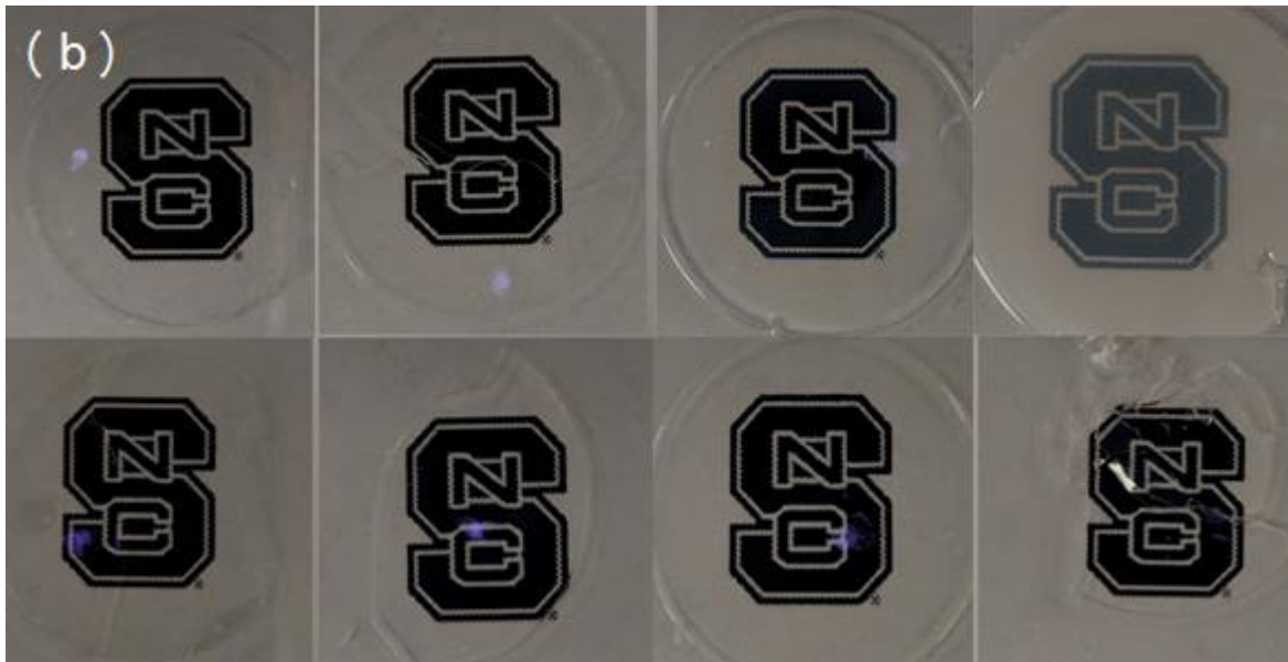
Figure 4.10. (a) Calculated turbidity values from UV-Vis spectrophotometry at a wavelength of 600nm. Reactive zirconia-containing systems are given by black squares, while passive zirconia-containing systems are given by red circles. (b) Images of 180µm-thick films on glass slides above NCSU logo. Top row, left to right: 50 wt% PDMS in MC, P25, P50, P75. Bottom row, left to right: R25, R50, R75, R80.
