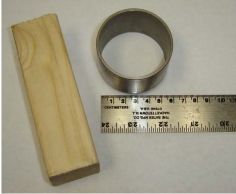
Figure 15 Soil bulk density measurement tools. Metal ring and wood block used to evenly distribute pressure delivered by hammer when pressing ring into the soil.
