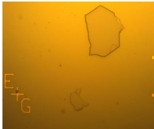
Figure 2-7: Optical image of an identified good quality flake after scotch-tape transfer method under 50x microscope zoom, to be used for defining top-contact layer using “KLayout” CAD tool.
