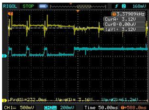
Figure 4-10 Wi-Fi module: initial state and steady state
