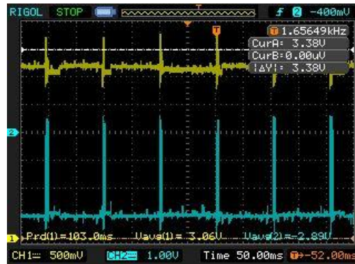
Figure 4-19 Wi-Fi module: one-reference-voltage mode with bands 3.397V to 3.185V
