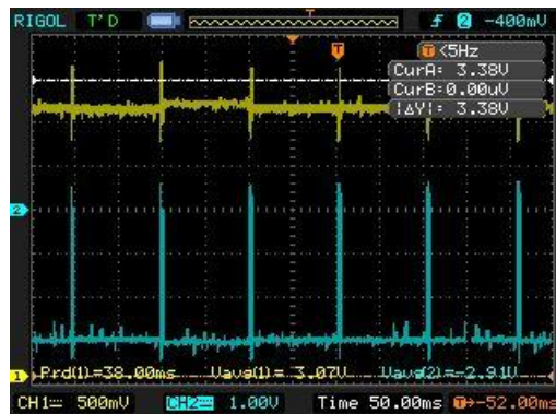
Figure 4-18 Wi-Fi module: two-reference-voltage mode with bands 3.373V to 3.208V
