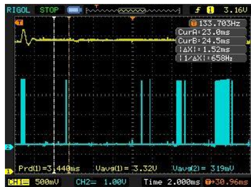
Figure 5-7 Periodical load in dead-band control: two-reference-voltage, dead bands 3.326V to 3.255V, zoom-out version
