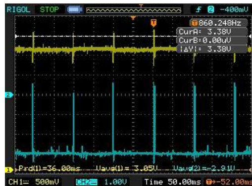
Figure 4-20 Wi-Fi module: two-reference-voltage mode with bands 3.397V to 3.185V
