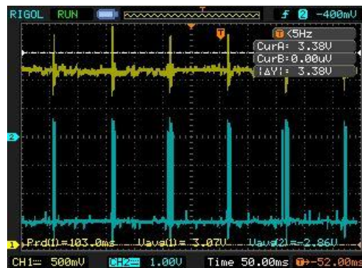
Figure 4-15 Wi-Fi module: one-reference-voltage mode with bands 3.350V to 3.232V
