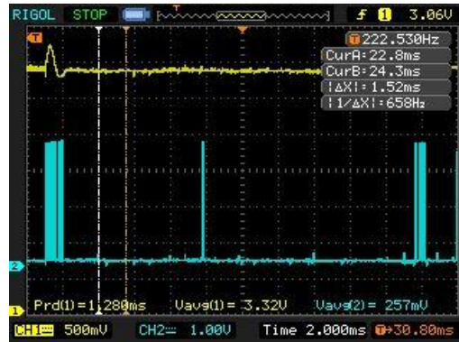
Figure 5-9 Periodical load in dead-band control: two-reference-voltage, dead bands 3.350V to 3.232V, zoom-out version
