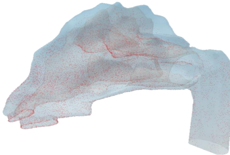
Figure 4. 26. Deposition pattern for 10 lpm flowrate and 1nm diameter particle.
