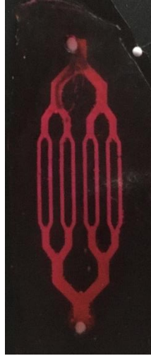
Figure 5-1 Phantom with 8 vessels with thickness of 500 \mu m and spacing of 1mm.
