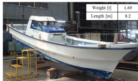
(a) The FRP boat used in the collision experiment
