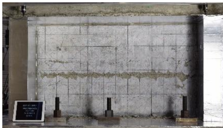
Photo 1. Final Failure (Specimen WM).
