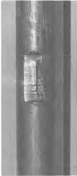
FIG. 1: Tube Failure Due to Fretting Wear
