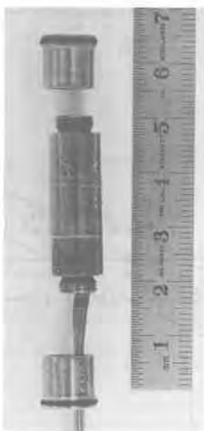
FIG. 10: Biaxial Accelerometer Probe for Tube Vibration Measurements
