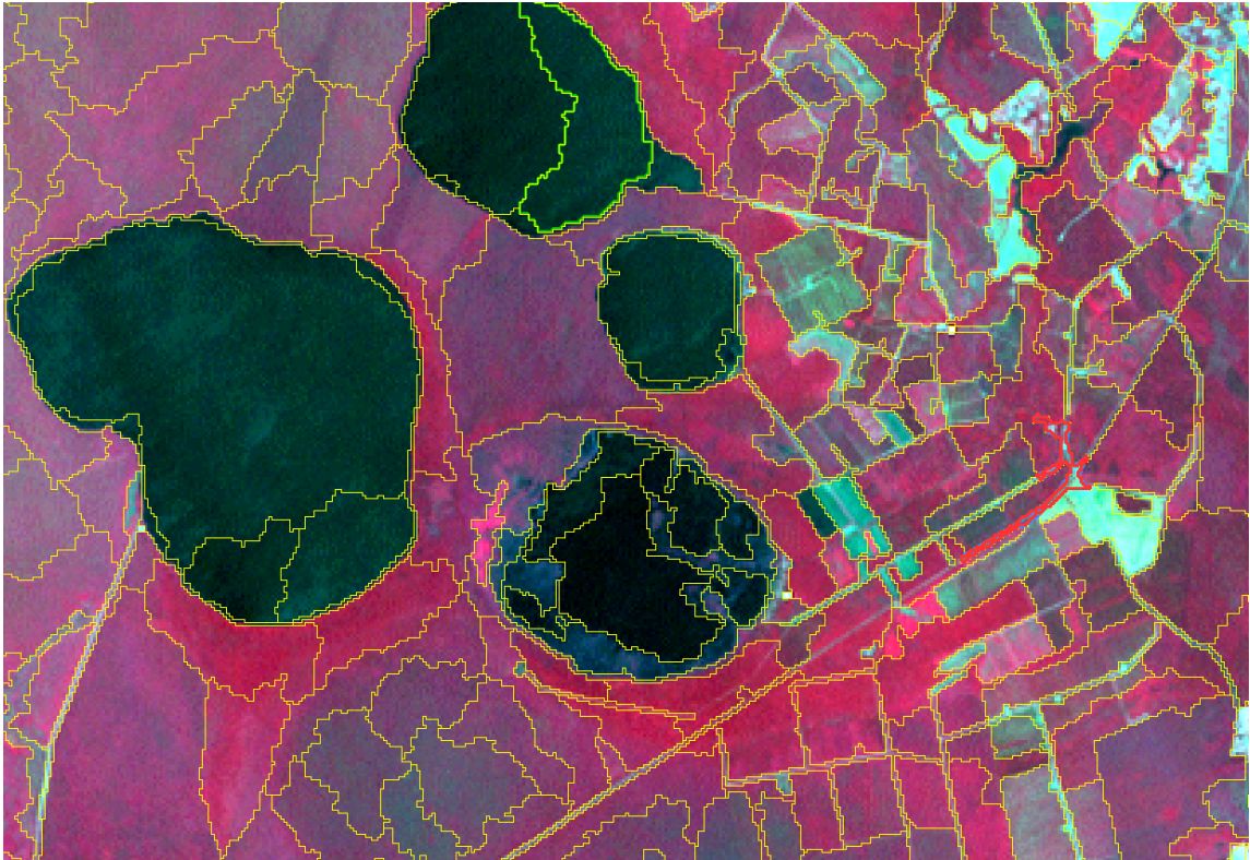
Figure 1.4. Image objects for a small area of the Croatan National Forest. Objects displayed over the Landsat TM image used to generate them. Image objects allow for hierarchical classification by incorporating data on both super-object and sub-object characteristics. In this case, shape index might be an important object level character, while variation of the pixels within an object, a sub-object characteristic, may be relevant as well.
