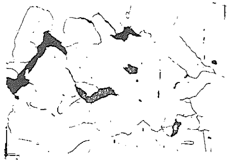
Fig. 11 - Intergranular decohesion on a specimen of AISI 316 H stainless steel deformed at 1300°C (magnification x 1000).
