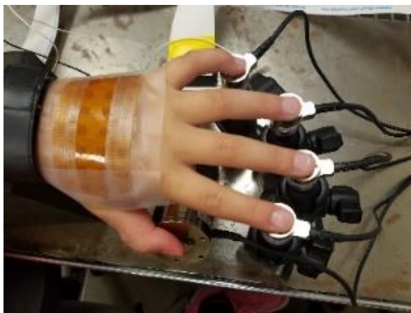
Figure 2.1: Participant's fingers resting on five 6-DOF load cells. The forearm is supported, and the wrist is in a neutral position. Digits were fully extended during testing.
