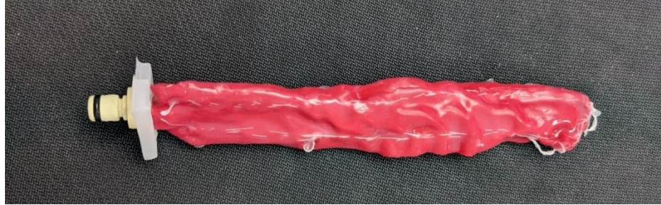
Figure 4.16: Composite Material Actuator. Lycra fabric embedded with DragonSkin 20.
