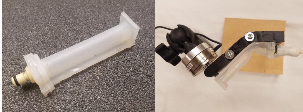
Figure 4.3: Actuator and Test Fixture. A) Semi-obround actuator with overmolded air connector. B) Actuator test setup with loadcell and jointed fixture.
