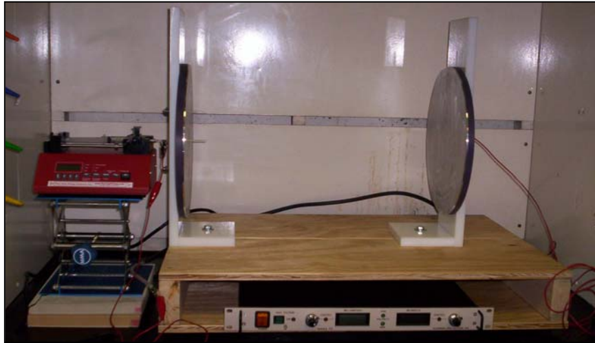
Figure 2.6: Picture of actual electrospinning setup.
