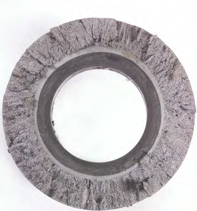
Fig. 14: Rough fracture surface of specimen
