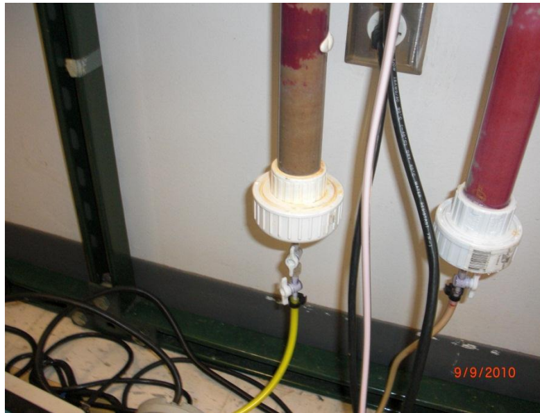
Figure 25-Image of weekly sampling, opening valves at inlet of column to start pumping of GW
