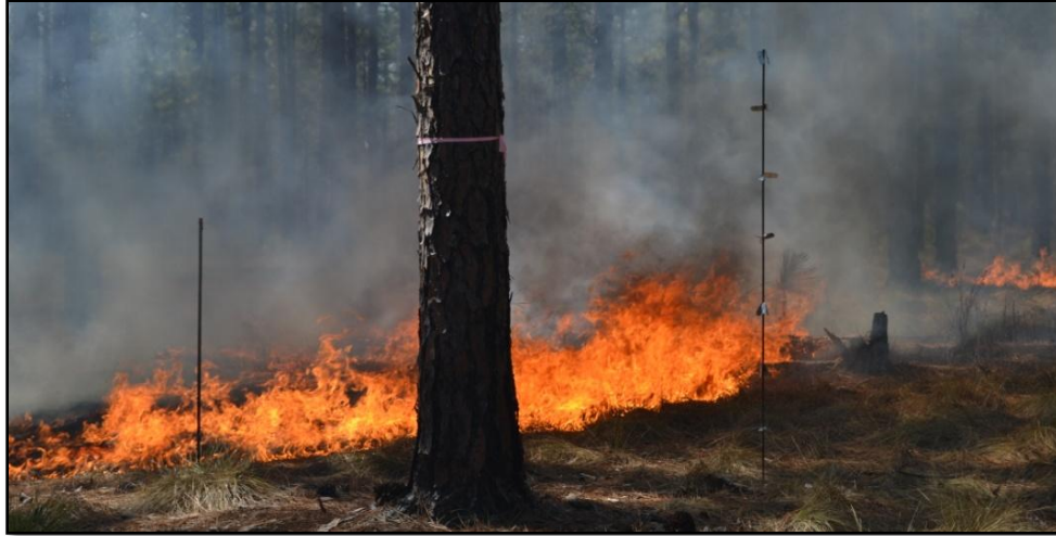
Figure 12: On right, rebar with tags painted with heat sensitive paints and located at 8 different heights, from ground level to 2.13 m. On the left, 1.52 m pole installed at 3.05 m from rebar to estimate (ROS) and (FH).
