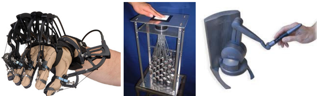
Figure 1.1. Examples of haptic interfaces including (from left to right) the CyberGrasp (photo: Wired), FEELEX (photo: University of Tsukuba), and Phantom Desktop (photo: SensAble Technologies)
