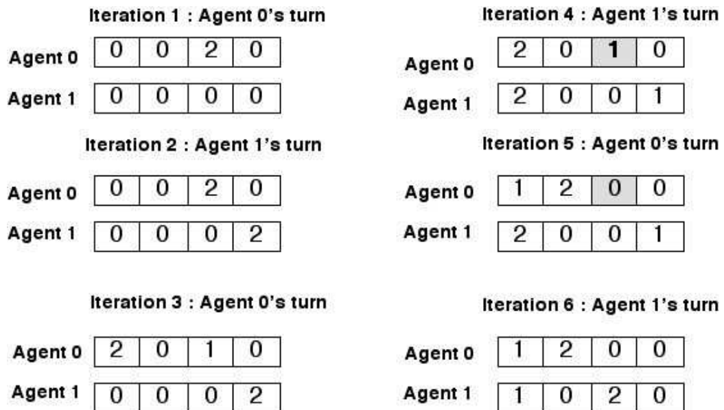
Figure 2.4: The status of the tabu list (attribute based memory) after each iteration for the search process shown in Figure 2.2.
