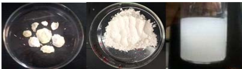
Figure 5.2.1. Photographic images of water-washed cellulose nanocrystals (left image), alcohol-washed cellulose nanocrystals (center image), and alcohol-washed cellulose nanocrystals dispersed in water (right image).
