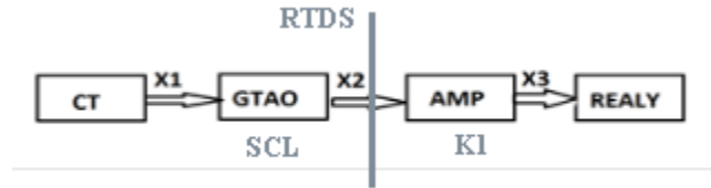
Figure 10 RTDS analog output setup from GTA0 card
