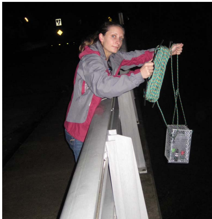
Figure A21: A student prepares to collect a sample by lowering the device into the creek below.
