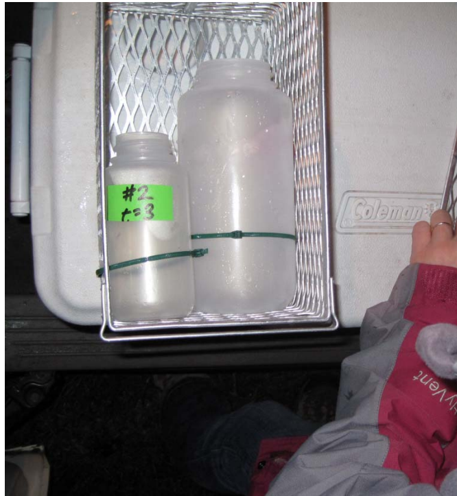
Figure A20: Detail of “bridge buddy” sample collection device being readied for use.
