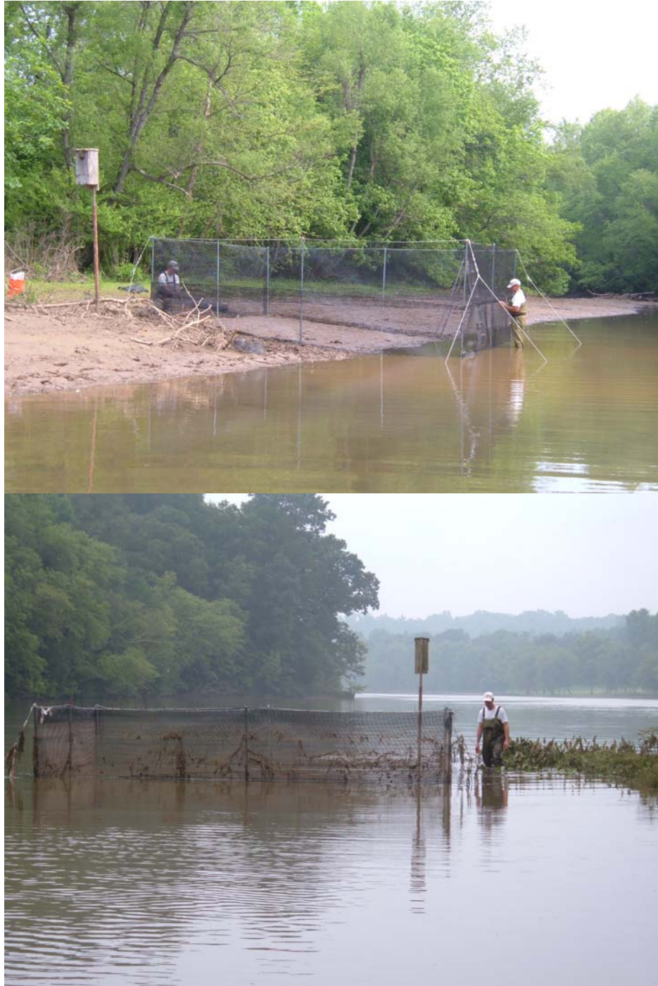
Figure 3. Experimental exclosures (6 m \times 6 m \times 2 m, 1.3-cm plastic mesh). The upper photograph was taken during exclosure construction with a 1-m drawdown of Lookout Shoals Lake. Lower photograph depicts normal lake level.
