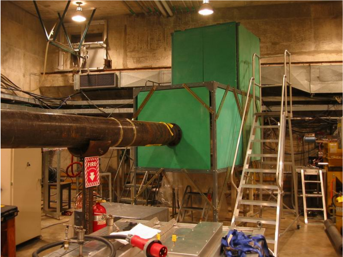
Figure 2-45. The assembly (include frame base, frame bell, polyethylene slabs, furnace table and two stairs).
