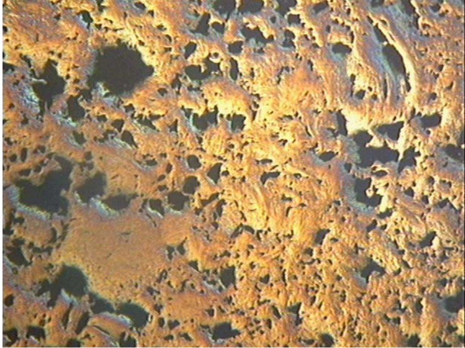
Figure 3-13. Reactor grade graphite sample surface picture taken by a scanning microscope at NCSU.
