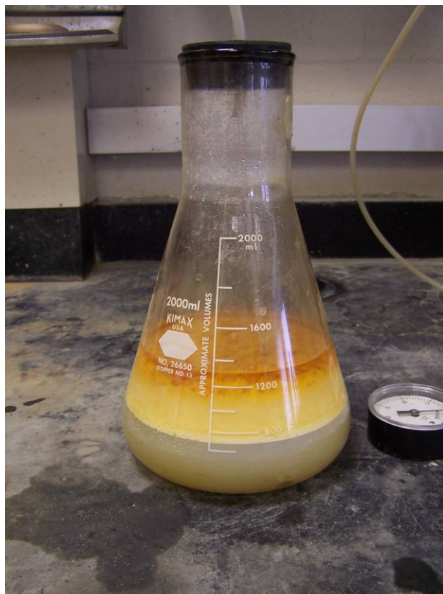
Figure 14. Erlenmeyer Flask Containing Biodiesel and Water After Equilibrated for 24 Hours, After 1 Hour Test
