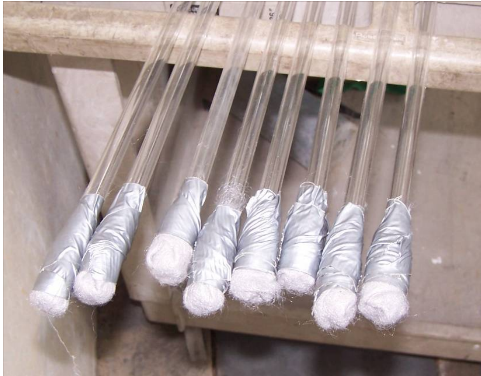
Figure 21. End Construction of Laboratory Piezometers for Setups 1 Through 3
