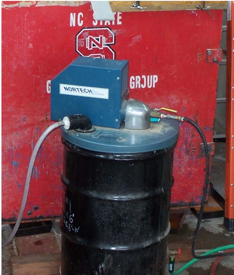
Figure 23. Vacuum Pump and Storage Tank Components of PVW Extraction System
