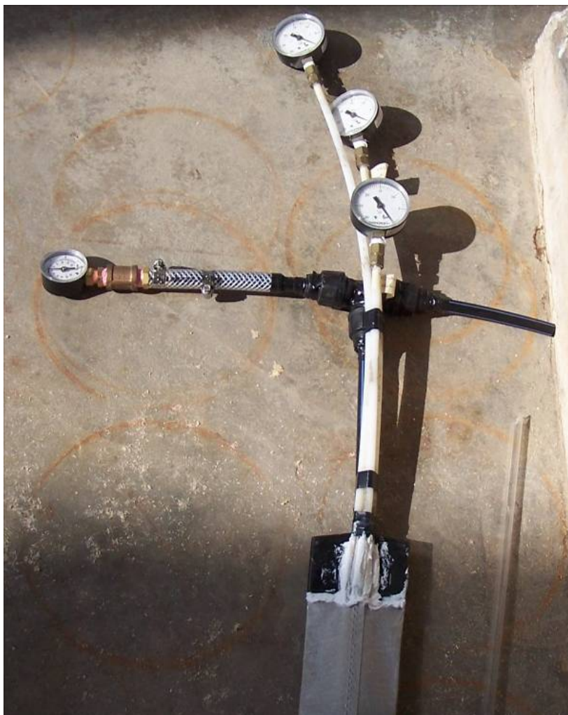
Figure 24. PVW Instrumented with Vacuum Gauges for Setup 1
