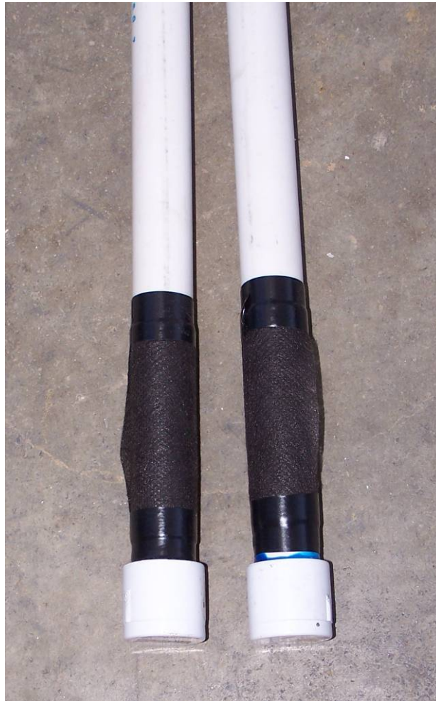
Figure 22. End Construction of Piezometers for Setup 4
