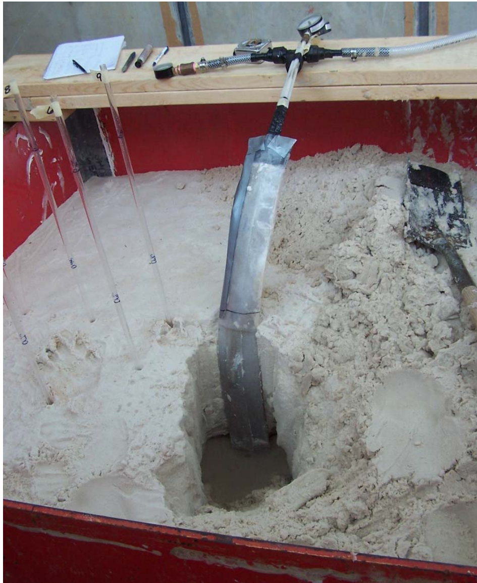
Figure 26. PVW in Sand Sample After Test Completion (Setup 1)
