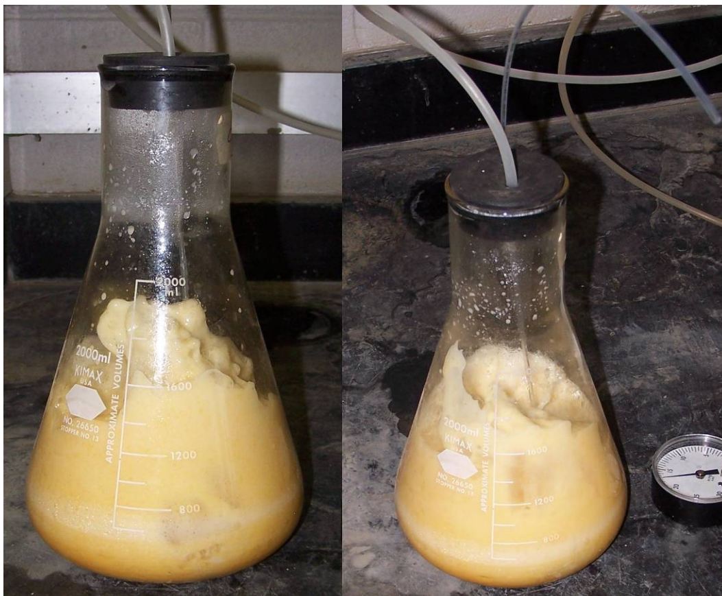
Figure 13. Mixing of 500 mL of Biodiesel and 1000 mL of Water by Applying 54.2 kPa Vacuum Pressure
