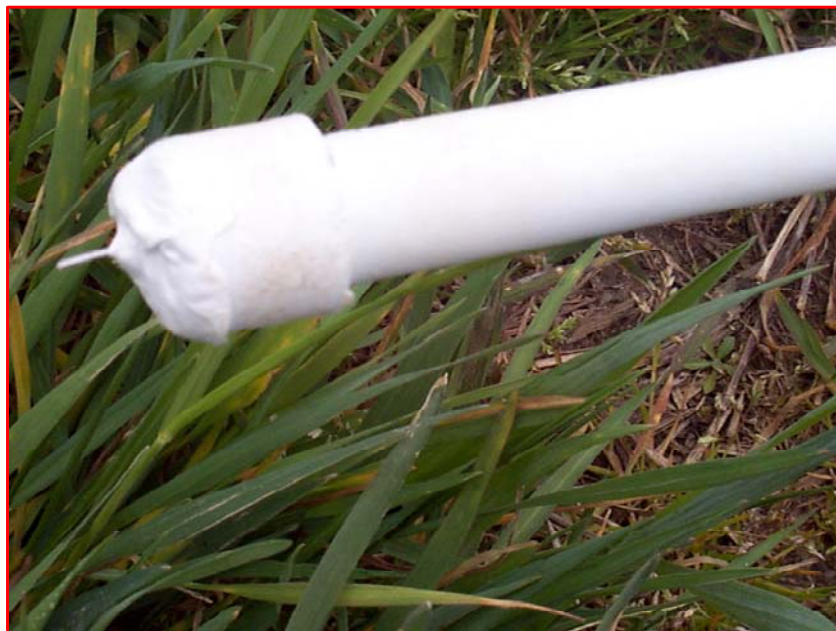
Figure 2.11 Protection of redox electrode
