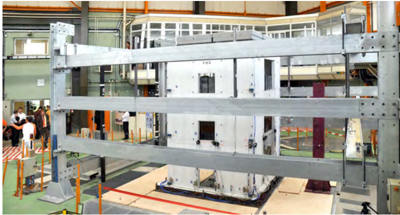
Figure 1. Photo of SMART 2008 structure and shaking table test setup (CEA).
