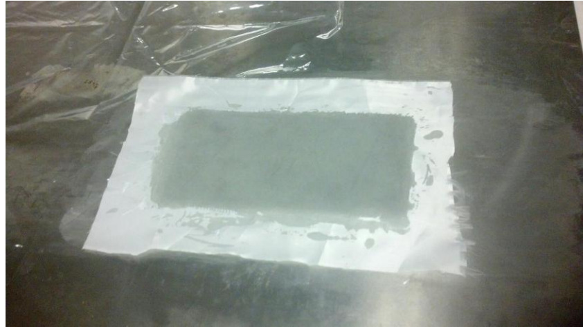
Figure 18: Peel Ply added to ensure nothing sticks to the fiberglass panel
