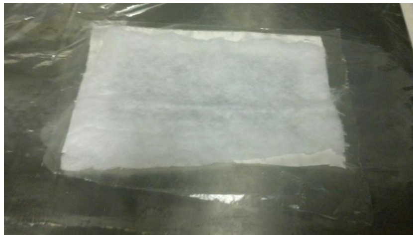
Figure 19: Breather and Bleeder added to the fiberglass panel to soak up excess resin
