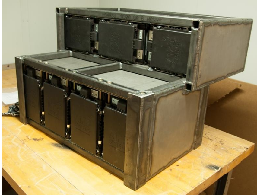
Figure 2: NCSU EcoCAR2 A123 battery pack
